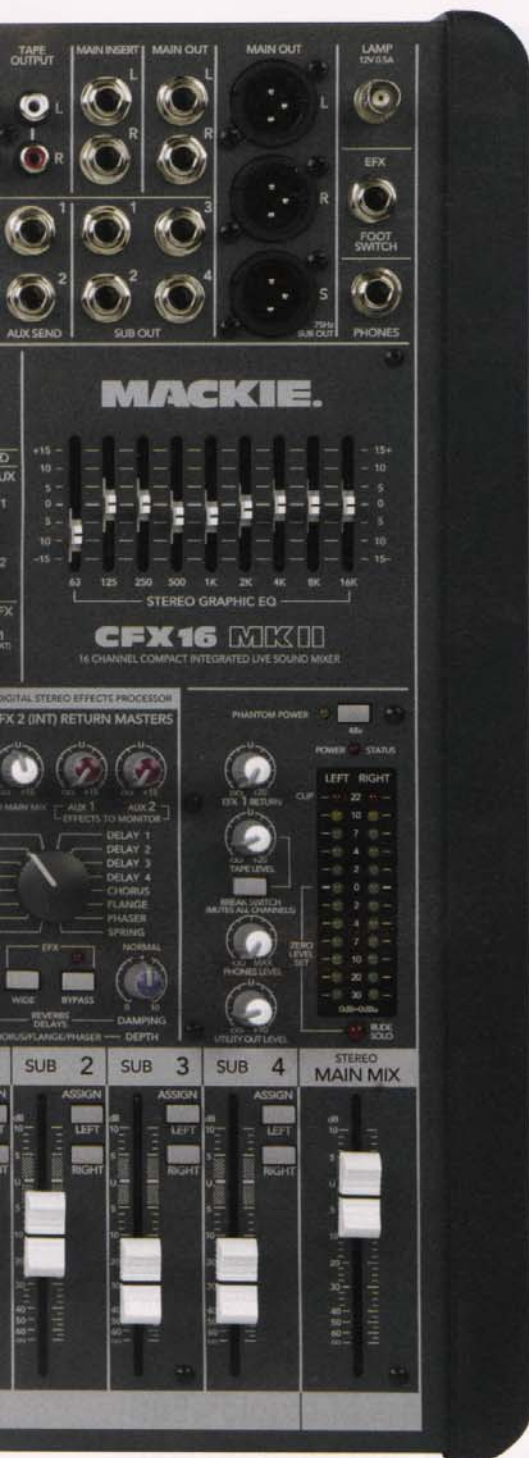
2 The 'master' connections panel, which includes the remaining ins and outs, plus a BNC lamp socket and a socket for connecting a footswitch to bypass effects.
