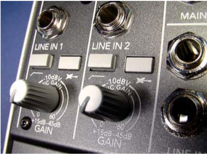
The two main inputs offer instrument in switches, lowcut filters, and plenty of gain.
