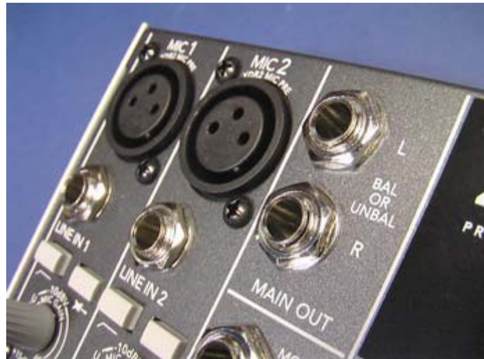
The first two ins accept either XLR or line/instrument ins. Also note the two 1/4" TRS outputs.
