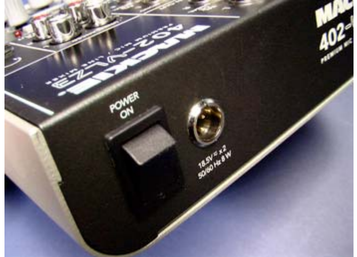
The locking connector could possibly save your gig, so don't underestimate its importance.
