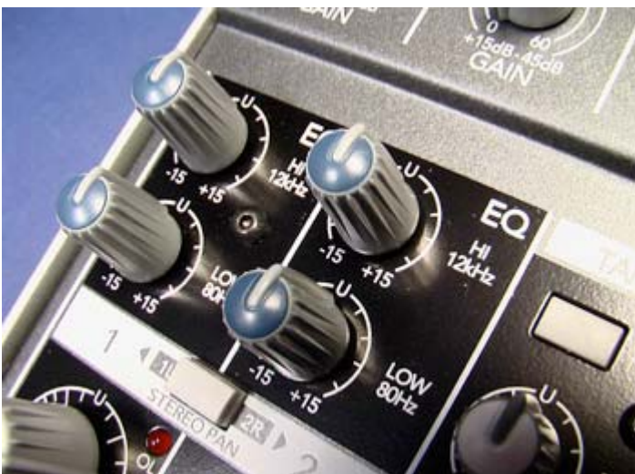
The two main inputs have two-band shelving EQ.
