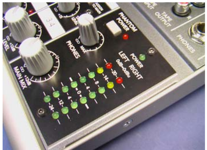
The two output meters use eight LEDs.
